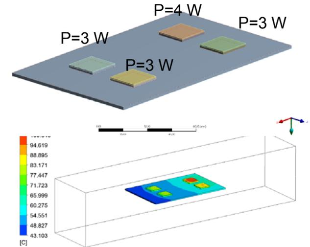
Temperature (PCB + Chips) in °C
