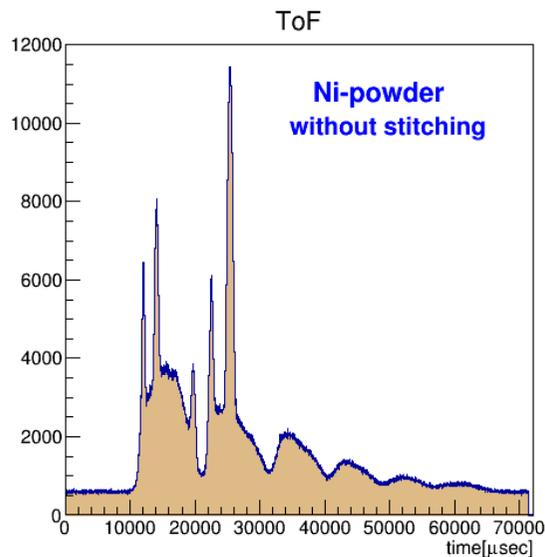
Raw ToF-spectrum only with  $T_0$  correction
