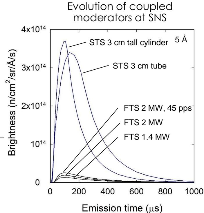
STS delivers the high flux and wide bandwidth required for time-resolved phenomena
