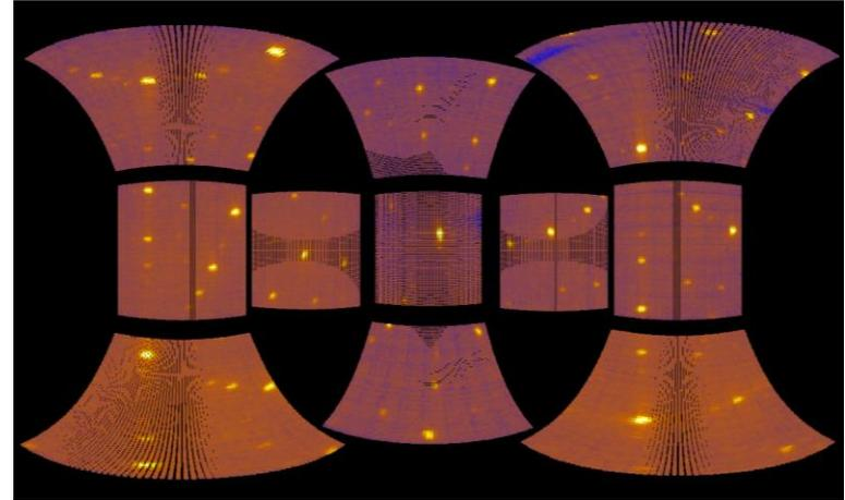
Low angle reflection, refraction and transmission from  $\text{Al}_2\text{O}_3$
