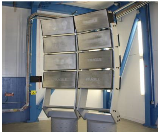
Eight modules installed on POWGEN stands
